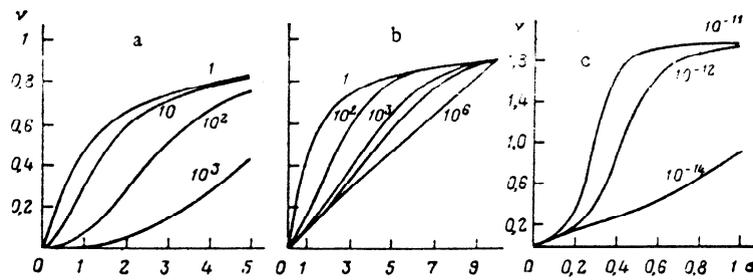
Fig. 1. Substrate activation of the rate of reaction (1). Here  $\nu$  is the dimensionless reaction rate described by Eq. (16), and  $\sigma$  is the dimensionless substrate concentration. The curves were plotted for various values of  $L$  (numbers on the curves) and  $n = 4$  (a, b), 10 (c);  $a = 0$  (a), 0.1 (b), and 200 (c); and  $c = 0.01$  (a, b) and 100 (c).
